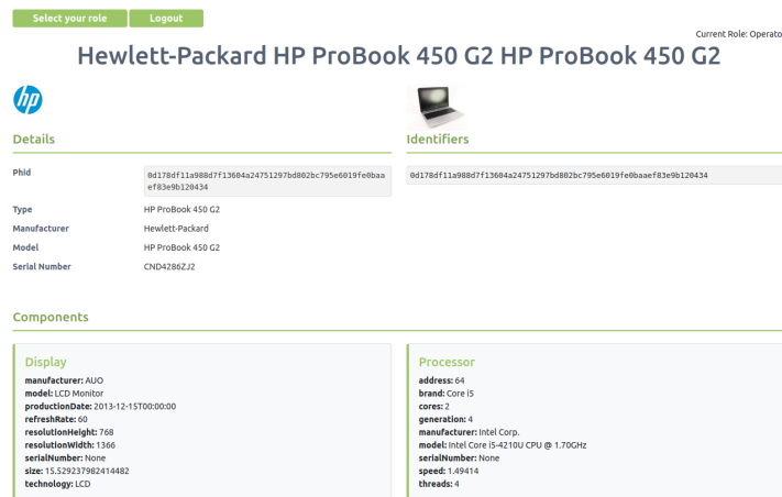
Fig. 5. Rendering of the product's DPP in HTML format delivered by the inventory service.
